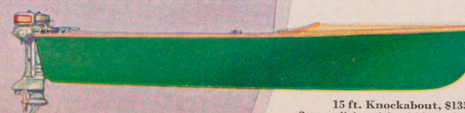
15 ft. Knockabout, $135 Strong, lightweight, 1/2 in. cedar planking, hollow and round construction; strong, bent white oak ribs sheer to sheer, round bilge bottom, 4 1/2 ft. beam.
