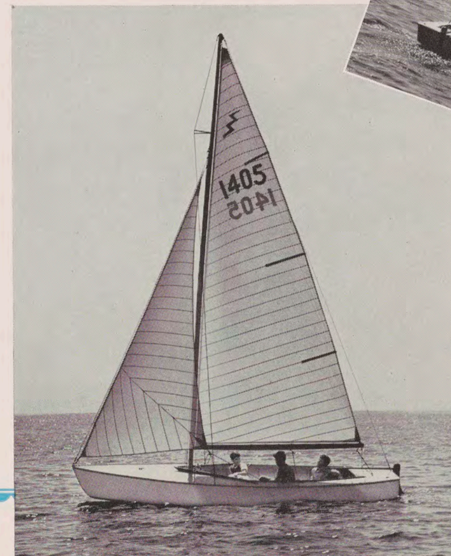
● At bottom of page—see the distinctive character of her appearance. You'll like the graceful ends, the sheer, splendid freeboard and handsome rig. You'll like the aristocratic sail plan with its high fore triangle, permanent backstay, double jumper stays and spreaders.
