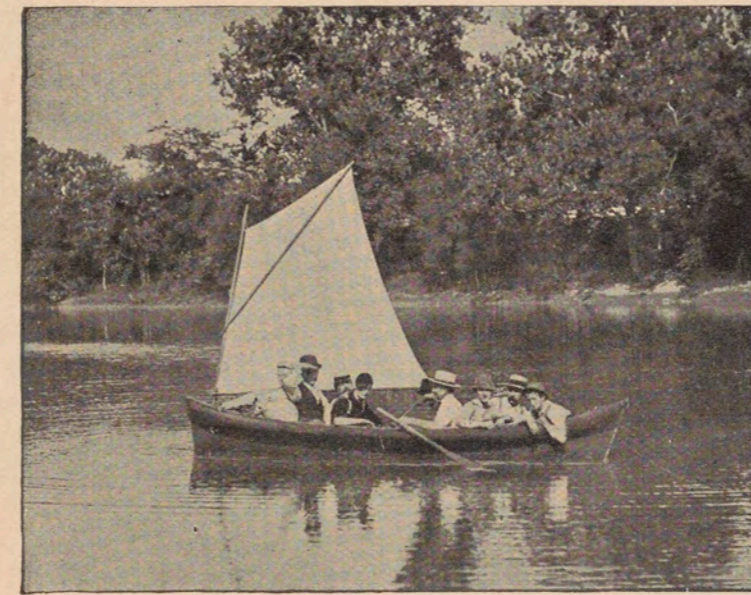
HALF-TONE FROM PHOTO OF 16-FOOT ACME, LOADED WITH 1300 POUNDS.
