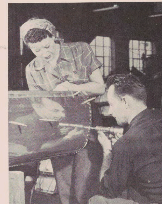
▲ After final riveting and finishing operations, another trim, new Aero-Craft Boat is ready to come off the production line.
