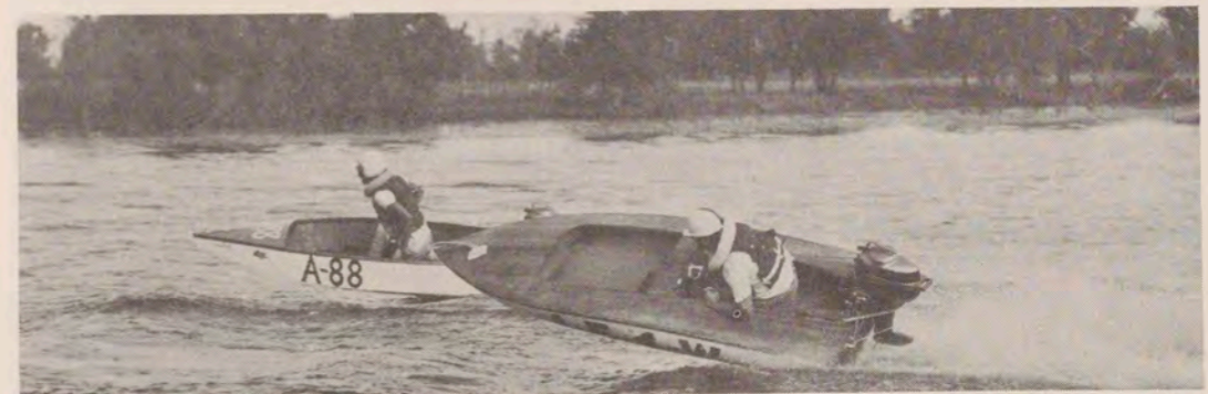
Runabouts, such as these BUs, are wild riding, slower than B Hydros but less prone to flipping. Their bottoms are monoplane design.
