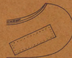
C. Patch applied over hole (fabric gone).
