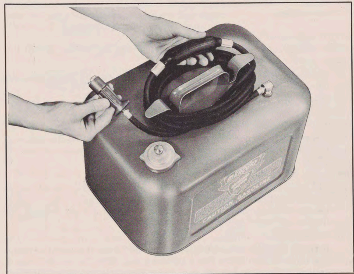
Figure 8 Remote Fuel Tank
