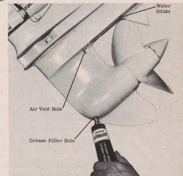
Figure 16 Lower Unit Lubrication
