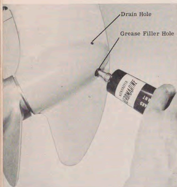
Figure 16 Lower Unit Lubrication
