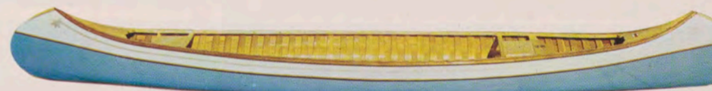
MOLITOR (Two-tone design shown.) Long decks, no thwarts required, outside stems, oval mahogany gunwales.
