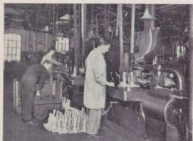
Pistons being machined, ground and honed by skilled mechanics on machines that ensure perfect accuracy.
