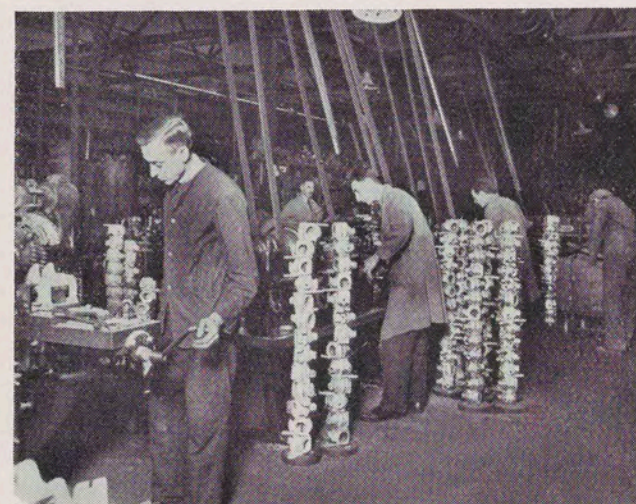
Cylinder cases machined and inspected.
