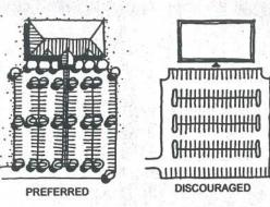
ORIENT PARKING AISLES PERPENDICULAR TO BUILDING ENTRANCES SO PEDESTRIANS WALK PARALLEL TO MOVING CARS
