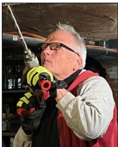
The process of dendrochronology requires taking a core sample from a piece of lumber.
