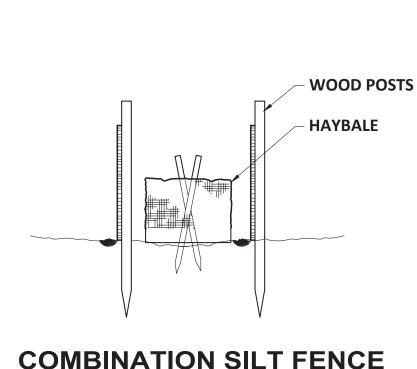
**COMBINATION SILT FENCE AND HAY BALE BARRIER** SCALE: "NTS"
