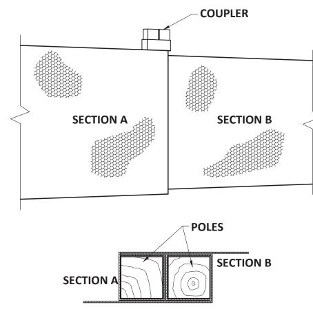
**JOINING SILT FENCE SECTIONS** SCALE: "NTS"
